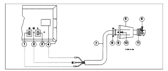
Figure 2-2. Connecting the Series 667xA Power Cord
